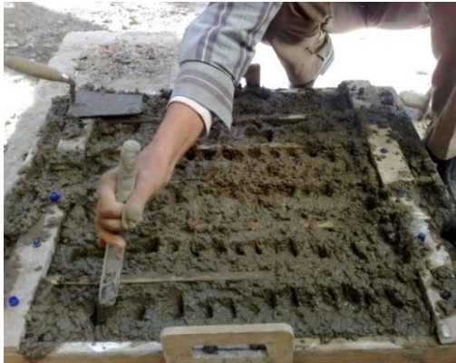
Figure (4): Compacting second layer.
