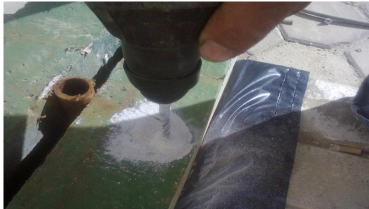
Figure (8): Taking specimens from the sample at a depth of 2.5 cm.
