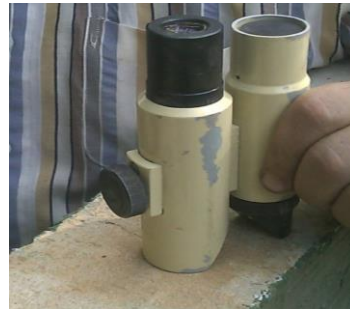
Figure (7): Crack width measurement.
